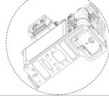
Slide the camera onto the baseplate until the stopper is bounced back, then fasten the
