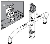
4. Attach the top arm to the two handles. To tighten, rotate clockwise .
