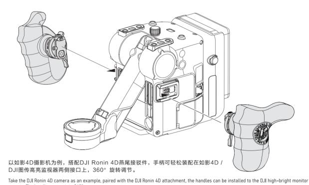
mounts. The handles can rotate 360°.
