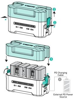
(1) Press and hold the lock buttons 1 on both sides to unlock, then remove the upper cover 2 .
