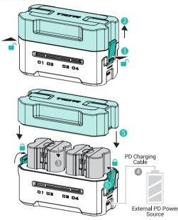
(1) Press and hold the lock buttons 1 on both sides to unlock, then remove
